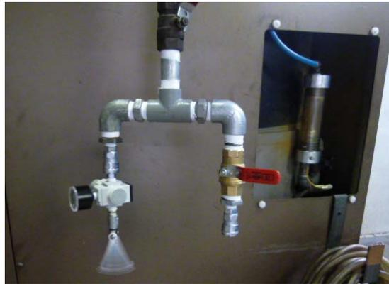
Pic.10. Durability Test (setting pressure : 0.6MPa)
