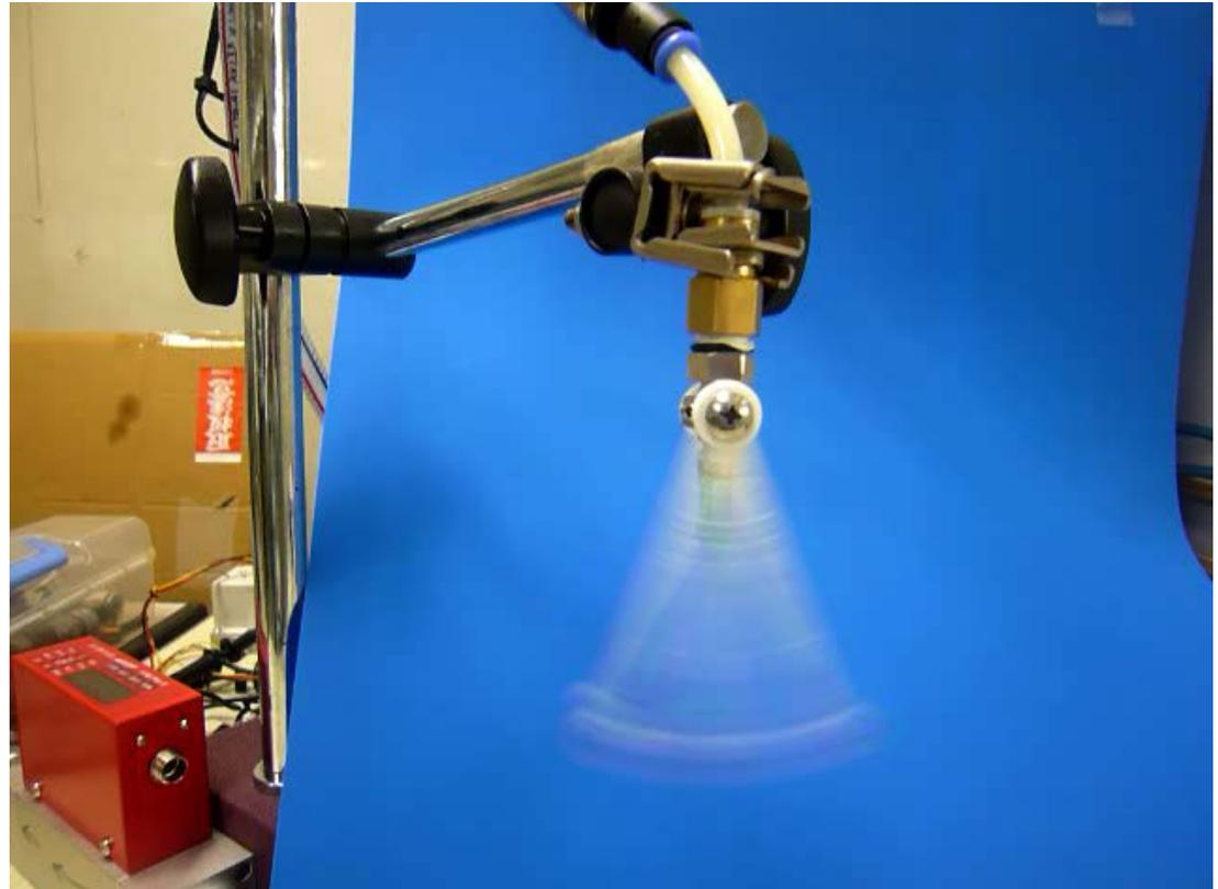
**Pic.1. Movement of the Mecha Swing Nozzle
