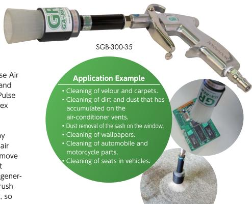
By combining the effects of the Pulse Air injected from a specialized nozzle and the brush vibration caused by the Pulse Air, the brush gun can clean complex parts such as circuit boards.
